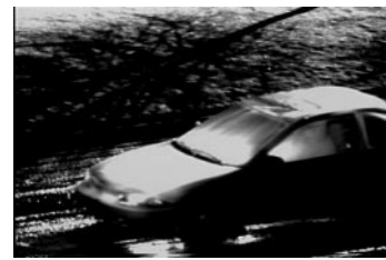
Fig. 5. Side snapshot of a fast-moving vehicle (65 mph) with a mid-infrared camera. The image appears heavily blurred, since the speed of the camera cannot keep up with the speed of the target
