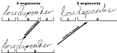
Fig. 14. Segment fusion for multi-segment shape recognition. An instance of the word *loudspeaker* with 3 segments is matched with an instance with 2 segments. The figure shows the correct segment fusion combination.
