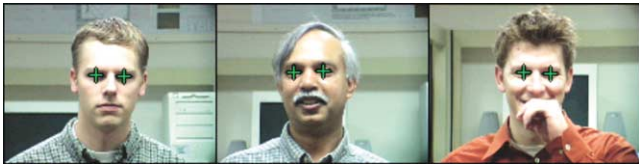
Fig. 29. Example output of the Identix FaceIT® face detector performing well on frontal faces. The locations of the eyes reported by the detector are marked with green crosses.
