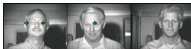
Fig. 28. Examples of our system having trouble due to failure of the template matching.
