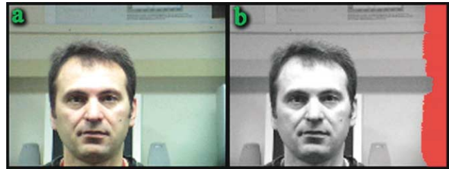
Fig. 10. An example of the integral projection in the visible band, (a) The visible band image, (b) The gray scale version of the visible band image with its integral projection overlaid in red. The dark stripe in the background creates a significant valley that would make eye detection very hard.
