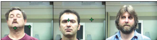
Fig. 30. Example output of the Identix FaceIT® face detector performing poorly on frontal faces. The location of the eyes reported by the detector is marked with green crosses.
