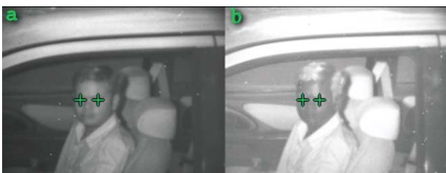
Fig. 32. Example of our system detecting the driver of a car in an outdoor environment. (a) Low near-IR image with the eye positions overlaid in green. (b) High near-IR image with the eye positions overlaid in green.
