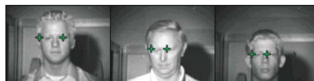
Fig. 27. Examples of our system having trouble due to failure of the integral projections.
