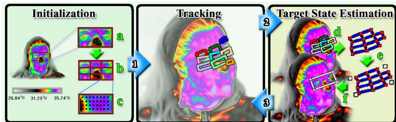
Figure 1: Overview of the tracking method. Initialization: consists of the following steps: (a) extraction of the user selected region of interest from the input video, (b) subdivision of the ROI into the tracking network, and (c) individual tracker template creation. Tracking: the individual trackers in the tracking network follow their targets. Target State Estimation: consists of the following steps: (d) the winning coalition is produced, (e) the deformation mesh is calculated from the winning coalition, and (f) the deformation mesh is used to calculate the target state. The method proceeds from initialization to tracking (arrow 1) to target state estimation (arrow 2) and back to tracking (arrow 3). In the latter transition, the winning coalition is passed back to the tracking stage to distribute the inter-tracker influence.
