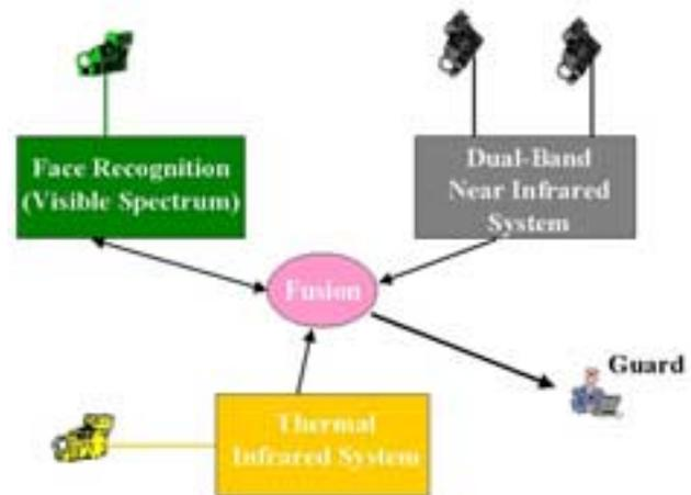
**Figure 16.** Architecture of a face/disguise detection and recognition system based on multi-band fusion.
