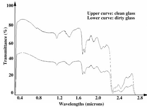
Figure 5. Transmittance diagram of a typical windshield.
