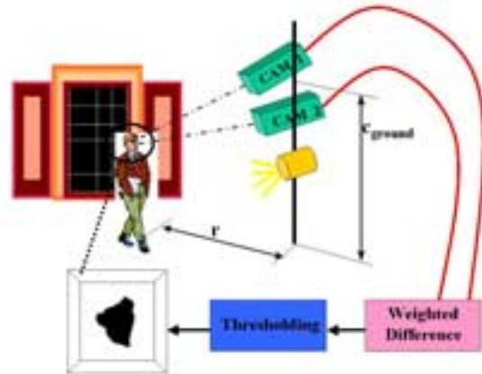
**Figure 6.** Architecture of the dual-band face detection system.
