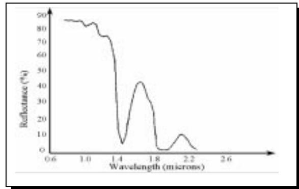
**Figure 5:** Reflectance of distilled water.
