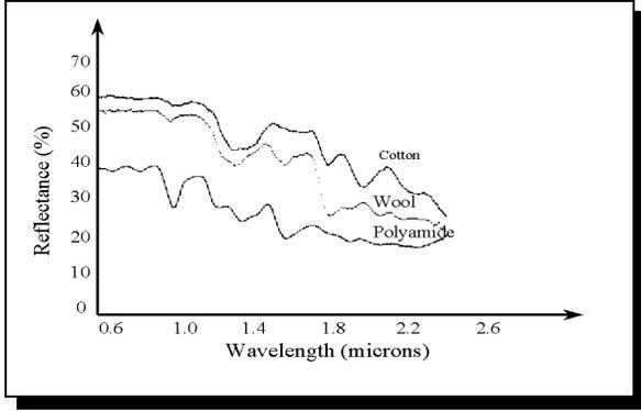
**Figure 6:** Reflectance of different fabric materials.
