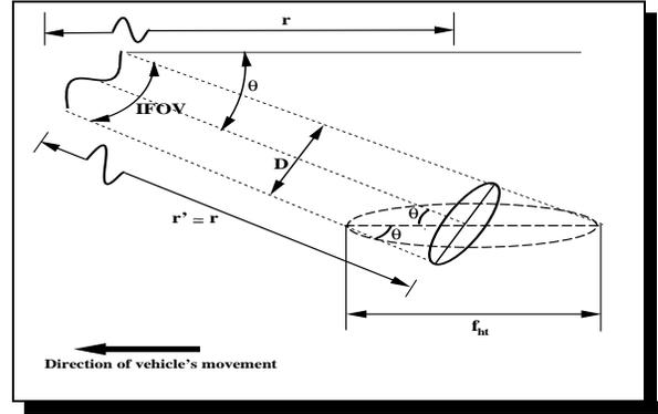
**Figure 8:** Geometry for the computation of a single pixel's horizontal translation - top view.
