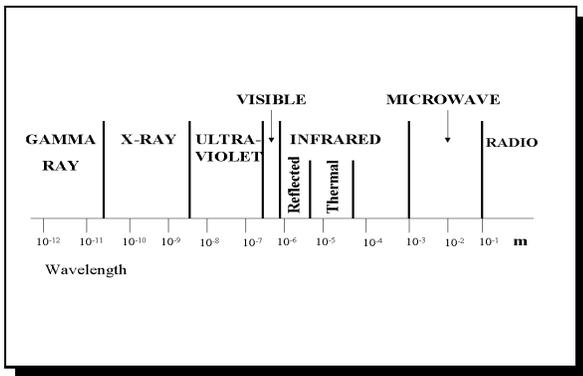
**Figure 1:** Electro-Magnetic (EM) spectrum.
