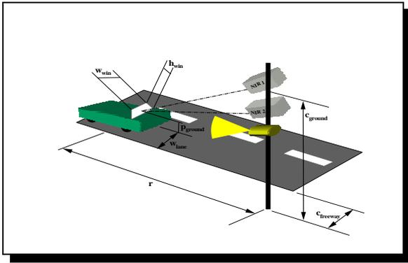
**Figure 7:** Configuration of the camera set.
