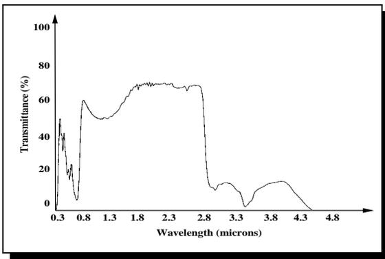
**Figure 3:** Transmittance of a typical tinted side-window.
