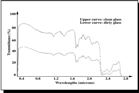
**Figure 2:** Transmittance of a typical windshield.
