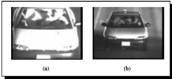
**Figure 9:** Near-infrared day time results. (a) Image in the band 1.1 – 1.4  $\mu m$ . (b) Image in the band 1.4 – 1.7  $\mu m$ .
