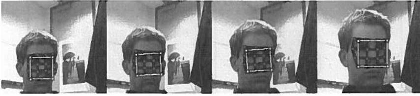
**Fig. 5.20** Example of tracking a face experiencing scaling and translation in the visual spectrum. The frames are shown chronologically from left to right. The deformation mesh is shown in blue, and the white rectangle represents the projected target state
