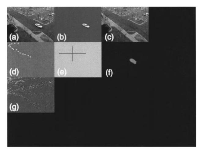
**Fig. 10.** Visualization of the computer vision operation of DETER. The snapshot was taken "live" on March 3, 2000. (a) Live video feed. (b) Segmented moving object. (c) Dynamically updated backgroud. (d) Trajectories of the current moving objects. (e) Centroids of the moving objects. (f) Results of the blob analysis. (g) Cumulative trajectory visualization of human and vehicle traffic for the past hour.
