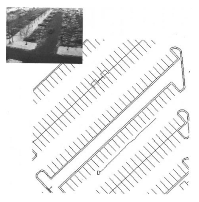
**Fig. 16.** Live video snapshot of a car moving out of the parking lot and its itinerary (line marked by the letter D) as it is recorded by DETER at the CAD design level.
