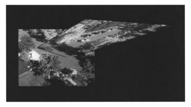
**Fig. 13.** Fused view from two DETER cameras. Because we compute a near optimal camera configuration scheme (coverage versus cost), the cameras are far apart and their optical axes form angles that vary wildly. As a result, one can notice the substantial image skewing produced by the highly nonlinear homography transformation. Despite the nonlinearity we achieve smooth image display thanks to a proprietary Honeywell warping algorithm.
