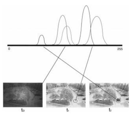
**Fig. 6.** Visualization of the mixture of normals model at the pixel level. The normals of a gray channel is depicted for simplicity purposes.
