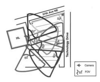
**Fig. 3.** Camera configuration scheme for DETER in the HL parking lot. This figure depicts the FOVs for the day channels of the cameras.
