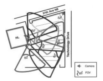
**Fig. 4.** Camera configuration scheme for DETER in the HL parking lot. This figure depicts the FOVs for the night channels of the cameras.
