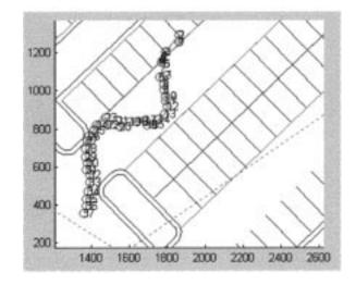
Fig. 15. An M-pattern traced by DETER. The centroids constituting the track are superimposed on the parking lot's CAD drawing. The M-pattern is a stroll mode favored by potential car thieves and it was one of the events staged during the benchmark recording.
