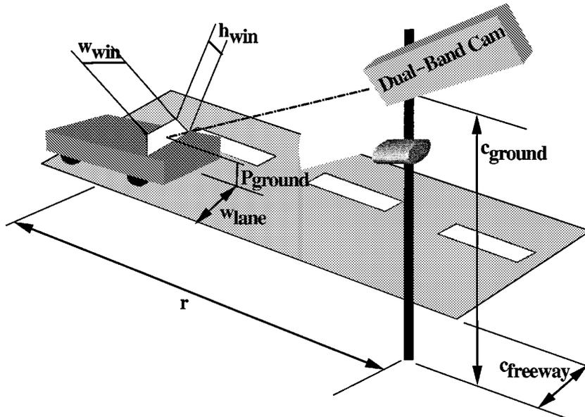
Fig. 10. Configuration of the camera set.
