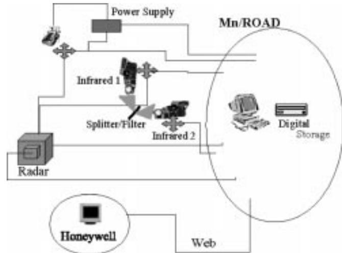
Fig. 16. Architecture of the prototype HOV counting system.
