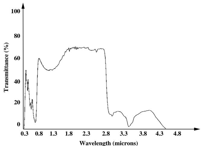
Fig. 3. Transmittance of a typical tinted side window
