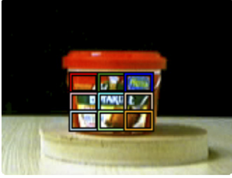
Fig. 2. Example of a 3 \times 3 tracking network on a visual image. Each tracker in the network is shown in a different color. Each tracker is tracking a separate part of the target. (For interpretation of the references to color in this figure legend, the reader is referred to the web version of this paper.)
