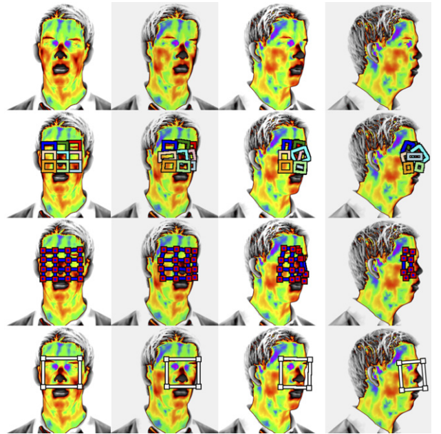
Fig. 6. Example of facial tracking in thermal video with a 3 \times 3 tracking network. The columns show progressive frames as the subject looks left. The second row shows the individual trackers in the tracking network. The third row shows the deformation mesh. The fourth row shows the computed target state.
