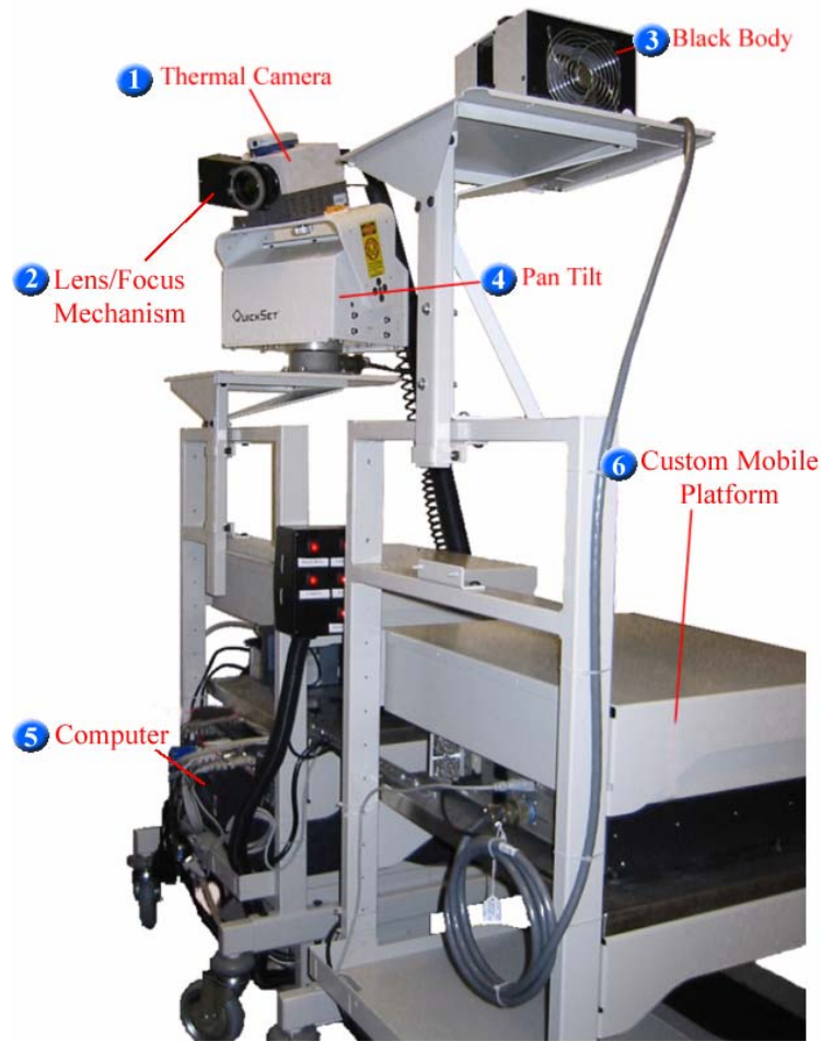
Fig. 1. The custom thermal imaging system used in our experiments.
