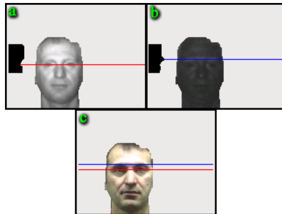
Figure 6: (a) The integral projection of the lower band skin region with the min location in red. (b) The integral projection of the upper band skin region with the max location in blue. (c) Both the min and the max locations overlaid on the visible band image for visualization purposes.
