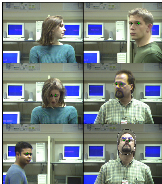
Figure10: Examples of the system's performance using rotated faces. The superimposed crosses indicate the locations of the eyes. The detection results have been overlaid onto the visible band image for visualization purposes only.
