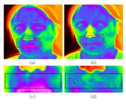
Fig. 1: The red boxes in (a) and (b) show the tracked region of the face in the first frame and the frame corresponding to the  $120^{th}$  second. (c) and (d) correspond to the tracked regions within (a) and (b) respectively. The black boxes within the tracked regions outline the region from which perspiration measurement is made.
