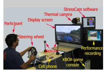
**figure 1.** Experimental setup; participant, imaging equipments, gaming equipments.
