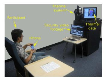
Figure 3. Experimental setup: Participant, imaging, and gaming equipment.
