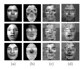
**Fig. 3.** The original (a) visible and (b) IR images followed by two different fused image results – (c) trained on a data set with lateral illumination and without glasses and (d) trained on a data set with glasses.
