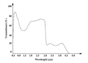
Figure 4. Transmittance diagram of a typical side window.
