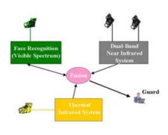
**Figure 16.** Architecture of a face/disguise detection and recognition system based on multi-band fusion.
