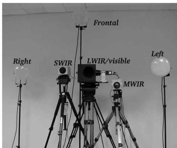
**Figure 6.3.** Camera and illumination equipment set-up used for simultaneous data collection of visible, SWIR, MWIR, and LWIR imagery.
