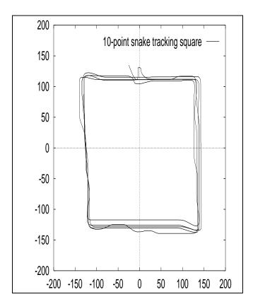
Figure 17: Tracking of a square target with the P & P algorithm (measurements in mm).
