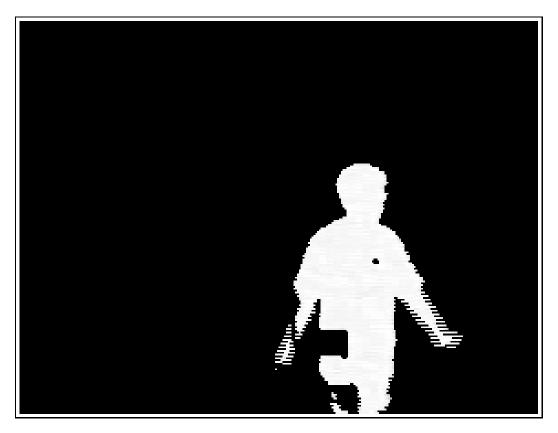
Figure 19: The difference image which provides image forces for the active deformable model.
