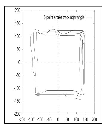
Figure 15: Tracking of a triangular target with the P & P algorithm (measurements in mm).
