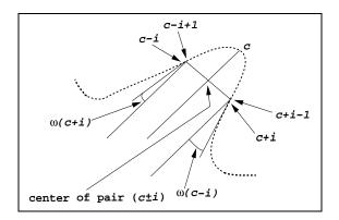
Figure 2: Geometric model for corner determination as proposed by Brault [6].
