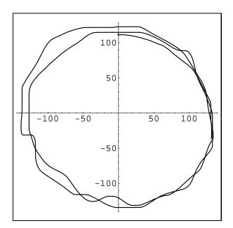
Figure 13: Tracking a rotating square target with an eight-point model (measurements in mm).
