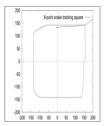
Figure 16: Tracking of a square target without the P & P algorithm. The target was lost after one revolution (measurements in mm).
