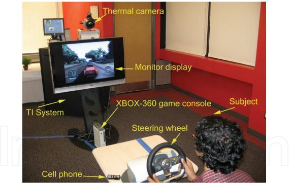
Fig. 3. Experimental setup; subject, imaging equipment, xBOX-360.
